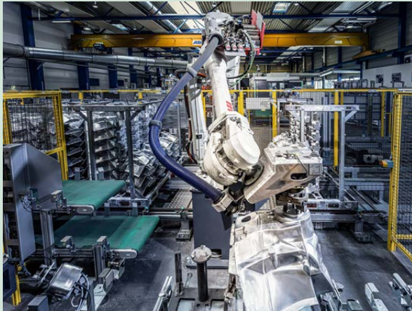
Automated high-pressure die-casting process at GF Casting Solutions in Altenmarkt (Austria)
