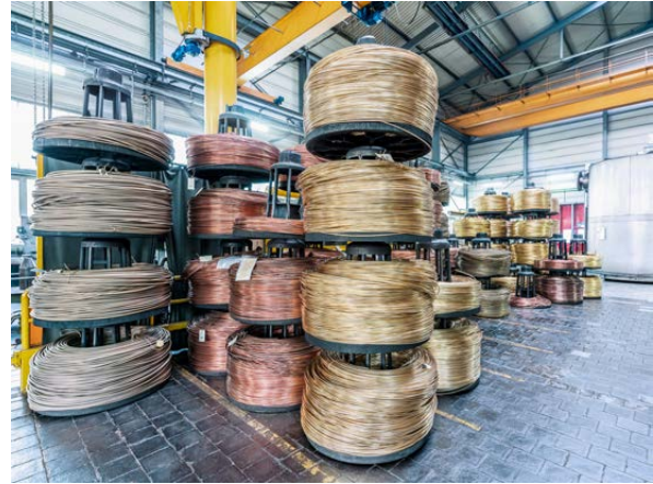
Copper alloy wire rods: primary material of EDM wire at Berkenhoff (Germany)
